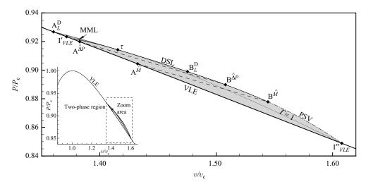
FIGURE 8. RSR for a polytropic van der Waals fluid with N = 20. The RSW with the maximum pressure difference and Mach number connects state points  $A^{\widehat{\Delta P}} B^{\widehat{\Delta P}}$  and state points  $A^{\widehat{M}}$  and  $B^{\widehat{M}}$ , respectively.
