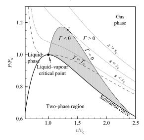
FIGURE 1. Liquid-vapour saturation curve (—) and the  $\Gamma < 0$  region (shaded region) for a BZT fluid in the volume-pressure plane computed from the polytropic van der Waals model with N = 2000. Selected isentropes (…) and the critical isotherm  $T = T_c$  (—) are also indicated. Note that the isentropes are concave down in the  $\Gamma < 0$  region. The isentrope  $s_{\tau}$  is tangent to the  $\Gamma = 0$  line in  $\tau$ .
