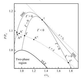
FIGURE 2. Selected pre-shock points  $A^D$ , A' and A'' along the isentrope  $s = \overline{s} < s_{\tau}$  for a van der Waals polytropic gas with N = 2000. Points I' and I'' are the intersections of  $s = \overline{s}$  with the  $\Gamma = 0$  curve. The vapour–liquid equilibrium (VLE) line is drawn together with the double-sonic locus (DSL).
