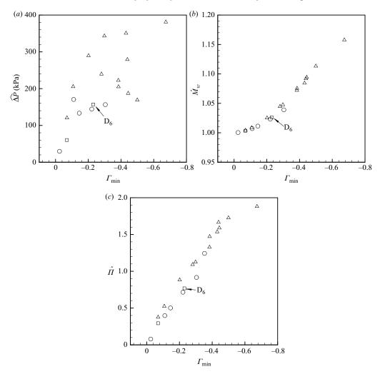
FIGURE 9. Maximum intensity of RSWs, calculated with the Stryjek–Vera–Peng–Robinson ( $\bigcirc$ ), Martin–Hou ( $\triangle$ ) and Span–Wagner ( $\square$ ) equations for the siloxane and perfluorocarbon fluids listed in tables 1. (a) Maximum pressure difference across an RSW, (b) maximum Mach number for an RSW and (c) maximum strength for an RSW.
